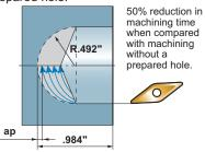
Machining a workpiece with prepared hole.
