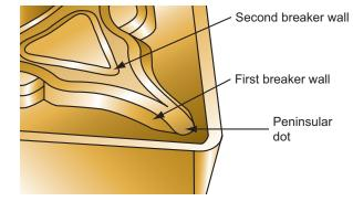
The large rake angle enables sharp cutting and excellent surface finish.
