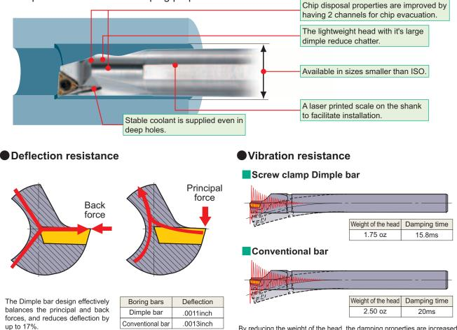
By reducing the weight of the head, the damping properties are increased.
