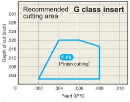
Cutting conditions Insert : CCGH21.51LF Cutting speed : 492 SFM
