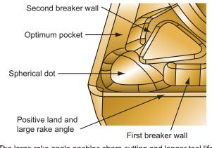
The large rake angle enables sharp cutting and longer tool life.
